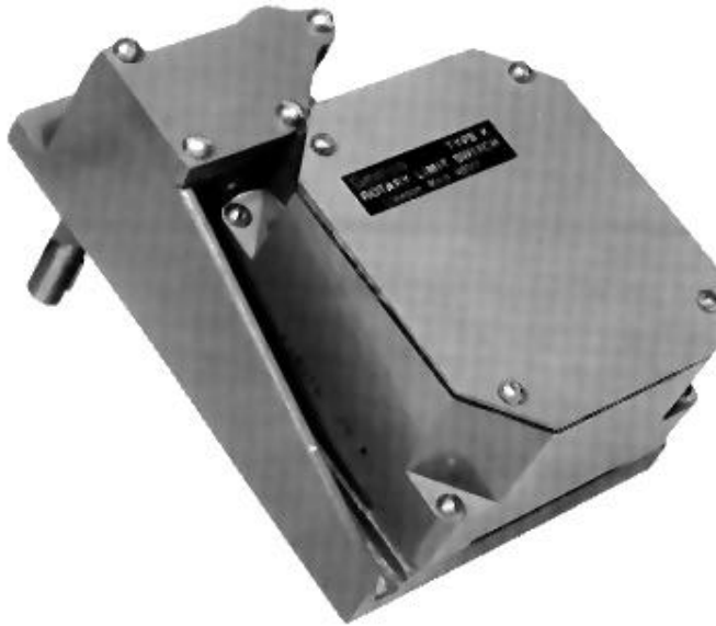
Two Circuit Rotary Limit Switch with a Special Mounting Bracket and Integral Right Angle Worm Gear for Mounting in a Power Jack.
